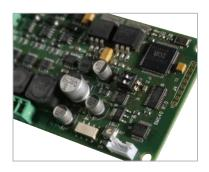
A special vector speed control function optimises efficiency and enables the micromotor to maintain a constant high torque throughout its speed range. Speed therefore remains constant even if the instrument is subjected to high torque loads. The compact electronic control card is composed entirely of SMT components. Dimensions: 98 x 58 mm. 32 VDC +/-5% - 500 mA.
